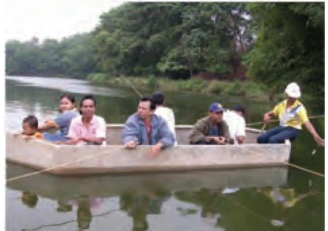
Figure 5 - The first-generation GRC boat
